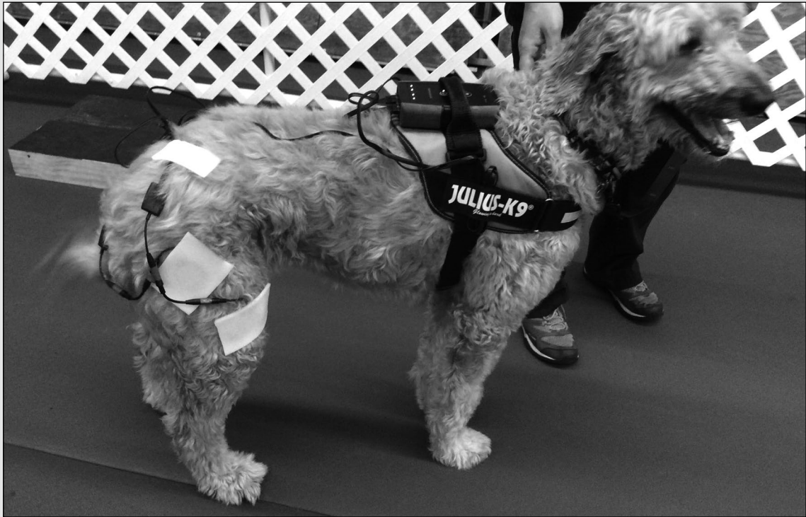
Figure 2. Dog wearing acoustic myography equipment.
